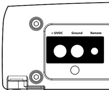
The G4500's “+12VDC” and “Ground” connections are designed to accept 4 AWG power wire. **4 AWG is a minimum power wire size for this amplifier.**
